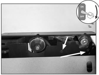
Figure 81. Lower blade guard removal.
